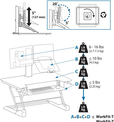
A+B+C+D ≤ WorkFit-T: 24.9 lbs (11.29 kg) WorkFit-TL: 29.9 lbs (13.56 kg) WorkFit-TLE: 29.9 lbs (13.56 kg) WorkFit-TX: 29.9 lbs (13.56 kg) WorkFit-Corner: 24.9 lbs (11.29 kg)
