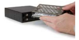
4. Slide the drive tray with installed hard drive back into the slot and close the door.
