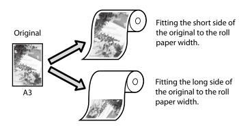
Select **Output Size** - **Fit to Roll Paper Width**, and then select whether to fit the short side or long side of the original to the roll paper width.
