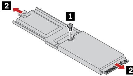
7. Install the new M.2 solid-state drive to the bracket **1** and tighten the screw **2**.
