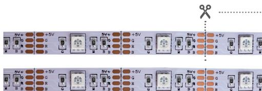
Each LED strip can be cut without affecting the use of the remaining strips.
