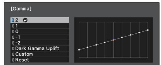
The larger the value, the lighter the dark portions of the image become, but bright areas may appear discolored. The upper part of the gamma adjustment graph becomes rounded. The smaller the value, the darker the bright portions of the image become. The lower part of the gamma adjustment graph becomes rounded.
