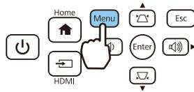
**2** Use the up and down buttons to select the item, and then press the [Enter] button to confirm the selection.
