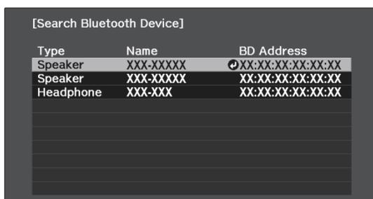
The next time you turn on the projector, it automatically connects to the last device it connected to. To change the connected device, repeat the procedure from step 5.
