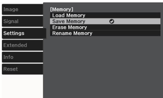
4 Use the up and down buttons to select the memory name you want to save, and then press the [Enter] button to confirm the selection.
