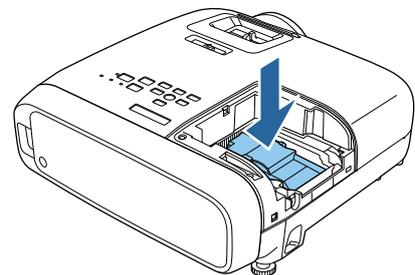
**7** Tighten the two lamp fixing screws.
