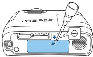
3 Pull out the streaming media player, and disconnect the USB power cable.
