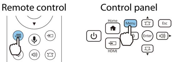
**2** Use the up and down buttons to select a mode, and then press the [Enter] button to confirm the selection.
