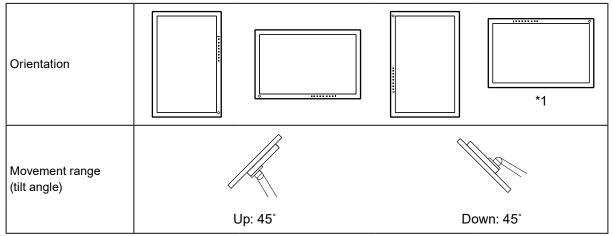
\*1 If you position the monitor facing in this direction, clean the power connector and the surrounding area regularly. If dust, water, oil, or other materials adhere to the device, it can cause a fire.
