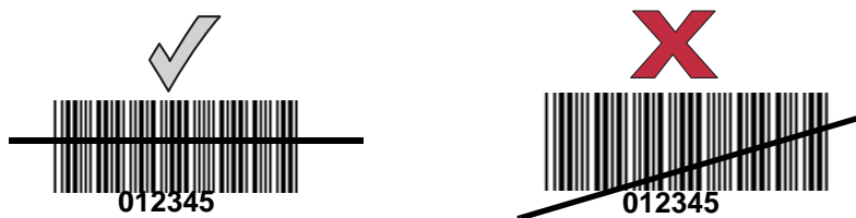
Figure 2-3 Acceptable and Incorrect Aiming
