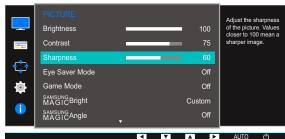
4 Adjust the Sharpness using the [▲/▼] buttons.
