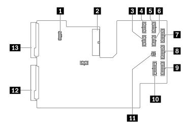
Figure 20. Connectors on the power distribution board
