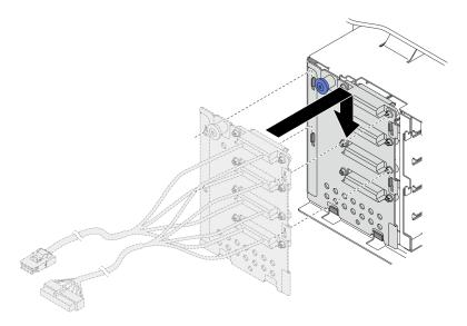
Figure 63. Installation of the 3.5-inch hot-swap drive backplate
