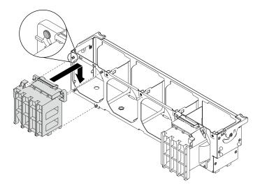
Figure 83. PCIe adapter holder installation
