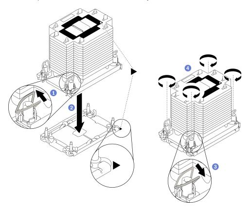
Figure 73. Installing a PHM
