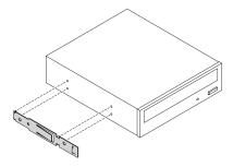
Figure 55. Optical drive retainer installation
