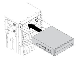
Figure 56. Optical drive installation
