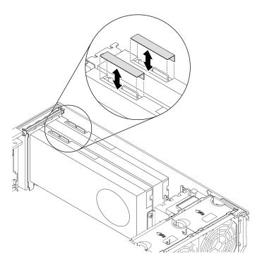
Figure 46. NVLink covers installation
