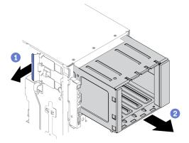
Figure 50. Expansion drive cage removal
