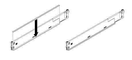
Figure 106. Applying left rail cover strip
