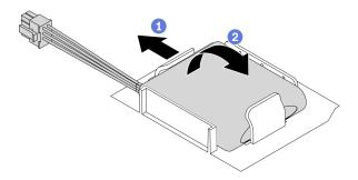
Figure 43. Flash power module removal
