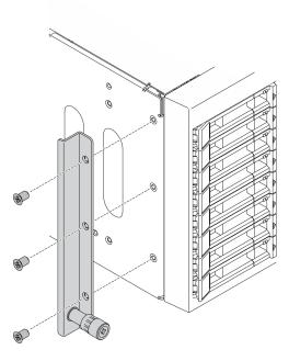
Figure 104. Installing left EIA bracket
