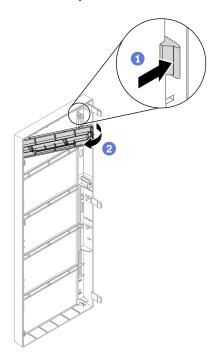
Figure 52. Drive bay filler cover installation
