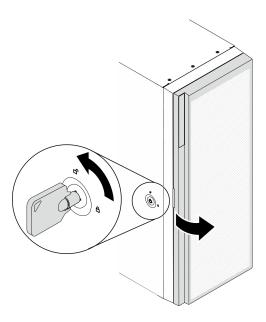
Figure 14. Server cover and front door lock
