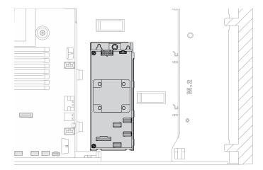
Figure 68. Internal CFF adapter location
