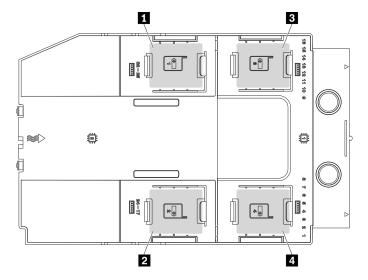
Figure 92. Flash power module slot location
