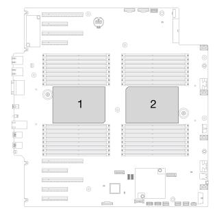
Figure 71. Processor locations on system board
