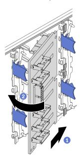
Figure 61. Installation of the 2.5-inch hot-swap drive backplane
