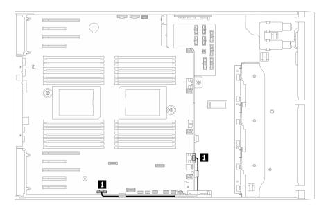
Figure 30. Cable routing to enable PCle slot 8
