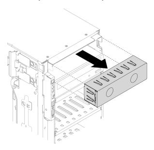
Figure 58. Drive bay filler installation
