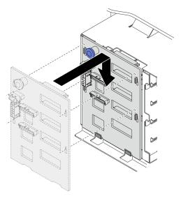
Figure 62. Installation of the 3.5-inch hot-swap drive backplane
