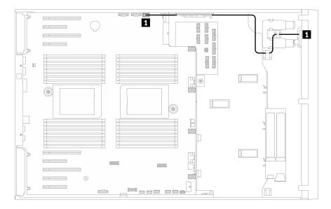
Figure 24. Cable routing for front panel
