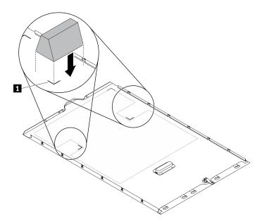
Figure 90. T4 filler installation
