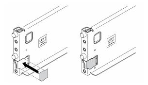
Figure 105. Applying left latch cover
