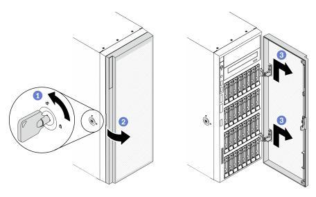
Figure 39. Front door removal
