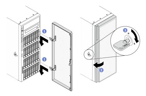
Figure 95. Front door installation
