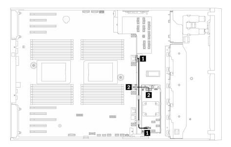
Figure 27. Cable routing for the CFF RAID adapter
