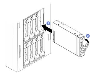
Figure 66. 3.5-inch simple-swap drive installation
