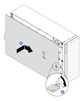
Figure 96. Server cover installation
