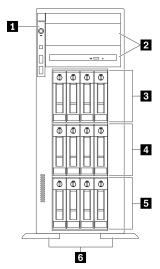
Figure 4. Front view of server models with twelve 3.5-inch simple-swap drive bays
