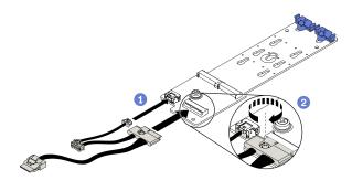
Figure 76. M.2 signal cable screw installation
