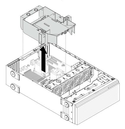
Figure 44. Air baffle removal
