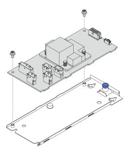
Figure 69. Internal CFF adapter tray installation
