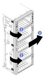
Figure 41. Front bezel removal
