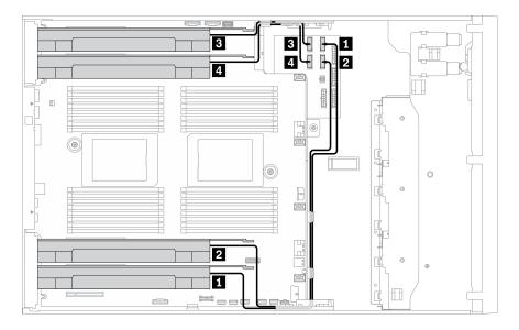
Figure 26. Cable routing for GPU
