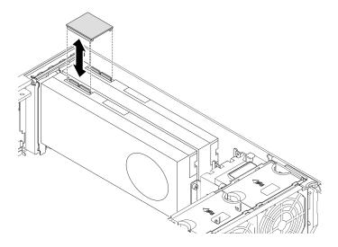
Figure 87. NVLink bridge installation
