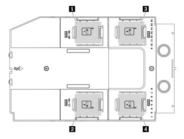
Figure 42. Flash power module slot location
