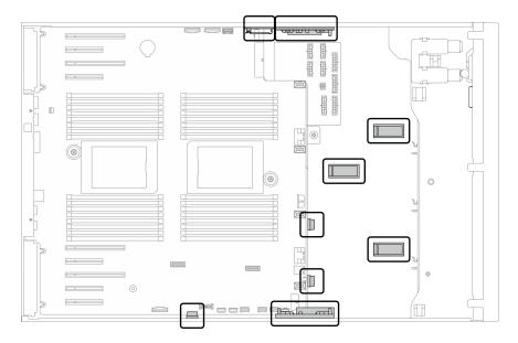
Figure 22. Cable clips and guides on 2.5-inch chassis
