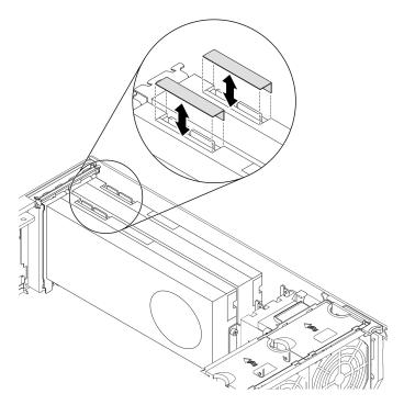
Figure 86. NVLink covers removal
