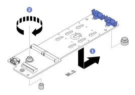
Figure 75. M.2 boot adapter installation
