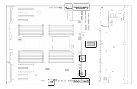
Figure 23. Cable clips and guides on 3.5-inch chassis
