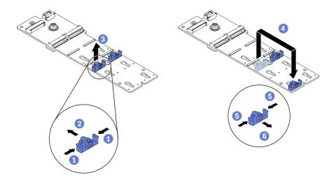
Figure 77. M.2 retainer adjustment
