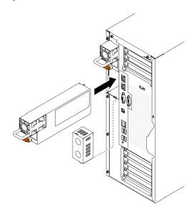
Figure 38. Hot-swap power supply installation
