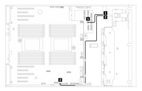
Figure 34. Cable routing for the USB tape drive
