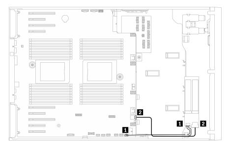
Figure 28. Cable routing for M.2 boot adapter
