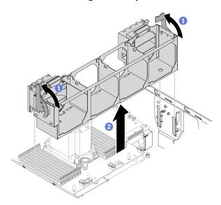
Figure 49. Fan cage assembly removal
