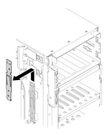
Figure 54. Drive retainer removal
