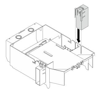
Figure 88. GPU filler installation
