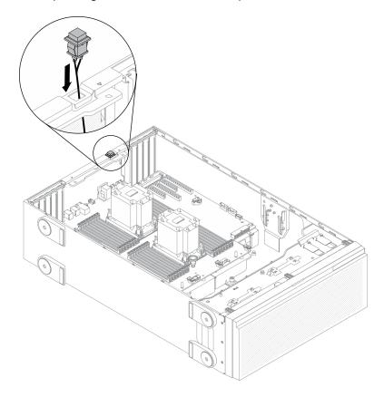
Figure 80. Intrusion switch installation
