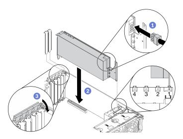
Figure 85. Full-length GPU adapter installation
