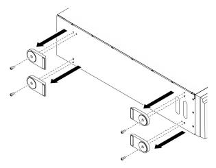
Figure 100. Removing foot stand
