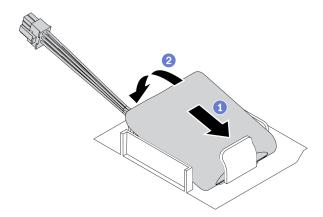
Figure 93. Flash power module installation
