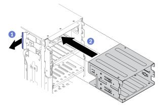
Figure 51. Optical drive cage installation
