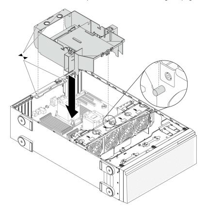
Figure 91. Air baffle installation
