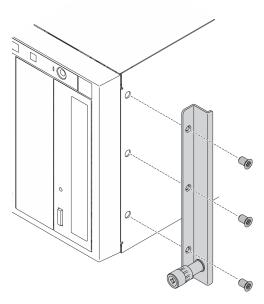
Figure 103. Installing right EIA bracket
