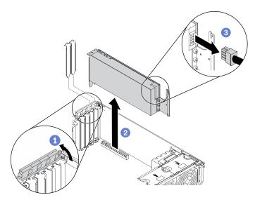
Figure 47. Full-length GPU adapter removal
