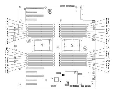
Figure 35. Processor and memory module layout
