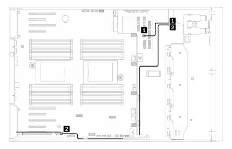
Figure 33. Cable routing for SAS tape drive to PCle slot 9
