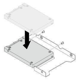
Figure 64. 2.5-inch drive installation to drive adapter
