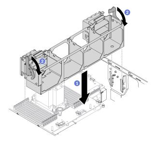
Figure 81. Fan cage assembly installation
