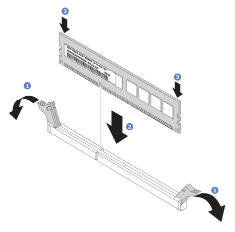
Figure 74. Memory module installation
