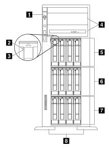
Figure 5. Front view of server models with twelve 3.5-inch hot-swap drive bays
