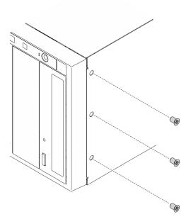
Figure 102. Removing screws on top of chassis
