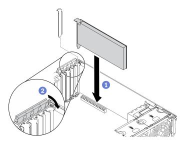
Figure 84. PCIe adapter installation
