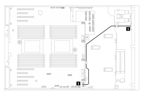
Figure 25. Cable routing for front USB
