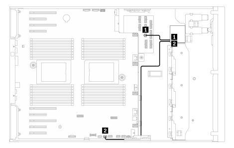
Figure 29. Cable routing for optical drive
