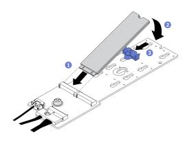
Figure 79. M.2 drive installation
