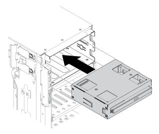
Figure 60. Optical drive installation
