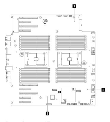
Figure 12. System board LEDs
