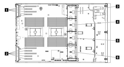
Figure 36. Fan slot locations
