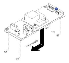
Figure 70. Internal CFF adapter installation
