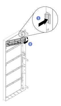
Figure 57. Drive bay filler cover installation
