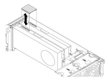
Figure 45. NVLink bridge removal
