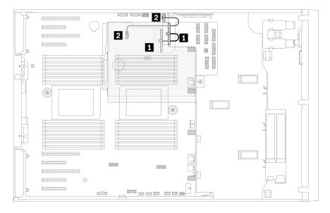
Figure 31. Cable routing for power distribution board
