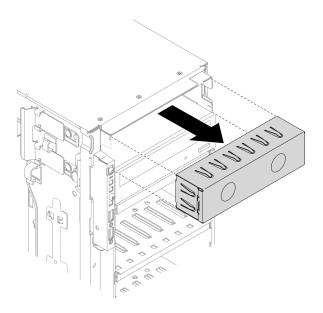
Figure 53. Drive bay filler installation
