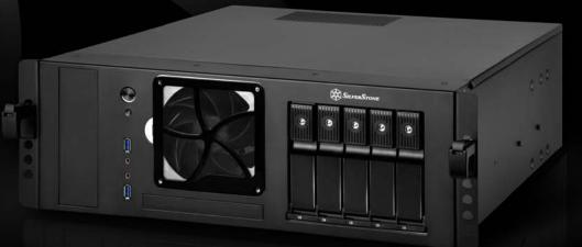
Magnetic fan filter included for easy maintenance against dust Supports graphics cards up to 13.78" (350mm) Supports ATX, Micro-ATX motherboards Support standard PS2 (ATX) up to 250mm Support five 3.5" SAS / SATA 6 Gbit/s drives with trayless & screwless design Adjustable drive status LED and fan control system
