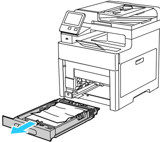
4. Remove any crumpled paper from the tray and any remaining paper jammed in the printer.
