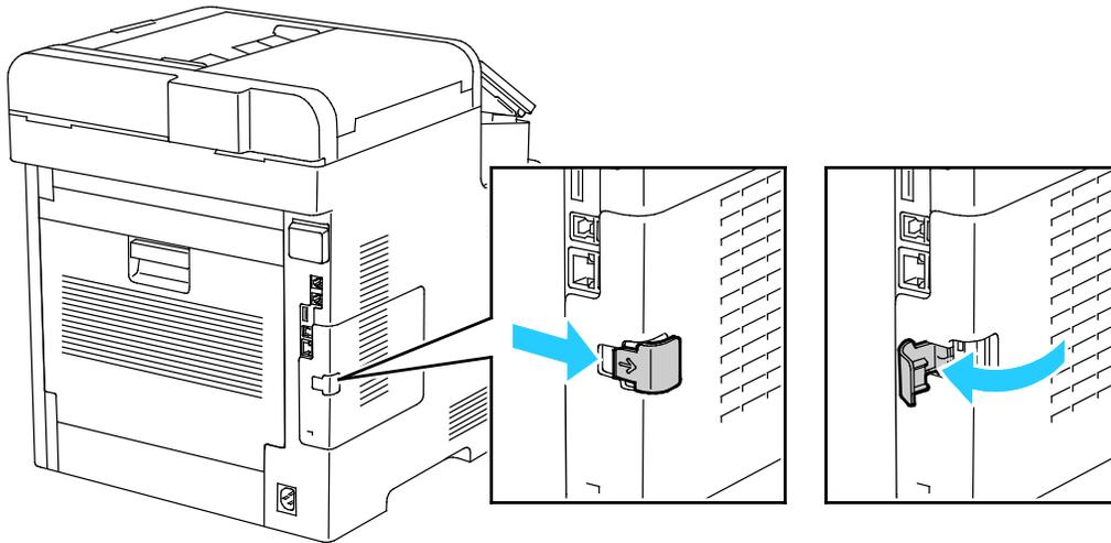
3. To remove the cover, slide it toward the back, then away from the printer.
