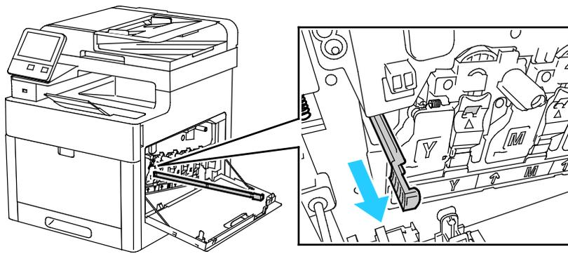
7. Insert the cleaning rod into one of the four cleaning holes until it stops, then pull out the rod. Repeat this two more times.
