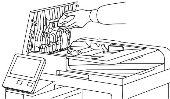
**Note:** If the feed rollers get stained with toner or debris, they can cause stains on the documents. To remove the stains, use a soft lint-free cloth dampened with a neutral detergent or water.
