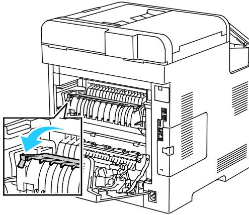
3. Remove any jammed paper from the back of the printer.
