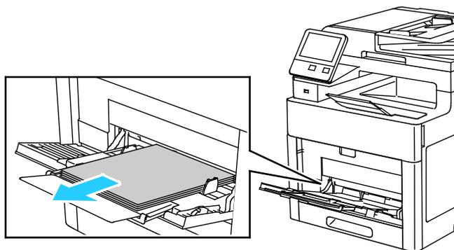
2. Grasp both sides of the Bypass Tray, then pull it straight out of the printer.
