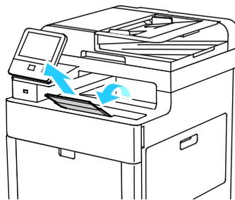
2. To print on longer paper, open the Output Tray Extension, then pull out the upper section until it stops.
