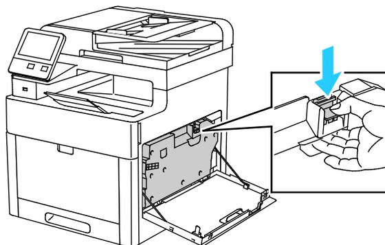
4. To remove the waste cartridge, lower the top of the cartridge, then lift it away from the printer. To prevent toner spills, keep the openings facing up.
