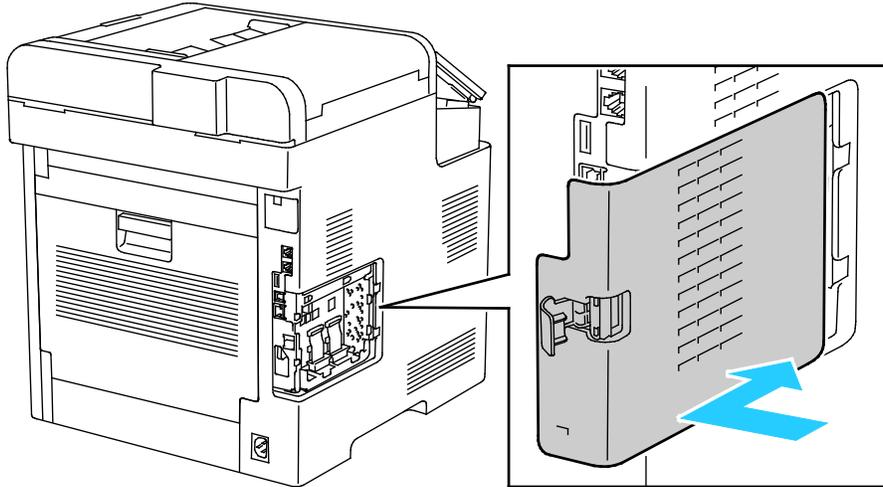
7. To latch the cover, swing the handle toward the front of the printer, then push the handle in until it clicks into the locked position.
