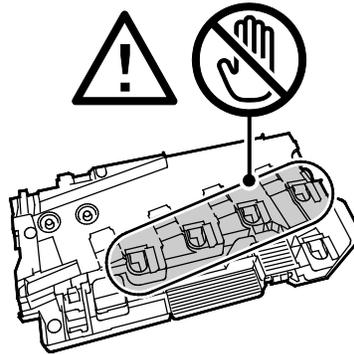
5. Place the removed waste cartridge on a level surface, with the openings facing up.
