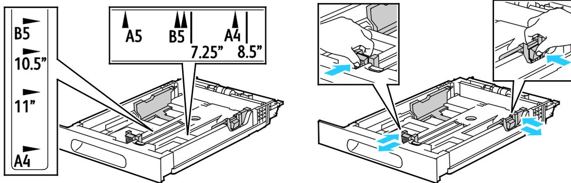
3. Load envelopes in the trays with the flaps closed, flap-side down, and the short edge leading into the printer.
