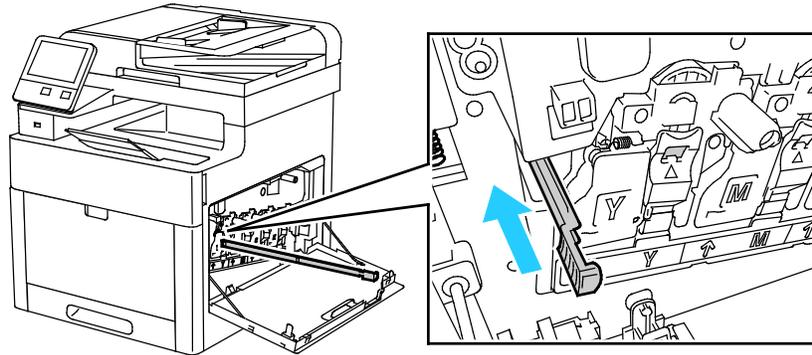
10. To reinsert the waste cartridge, lower the bottom of the cartridge into position. To lock the cartridge into place, push the top forward until the latch clicks into place.
