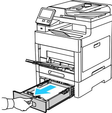
2. To remove the tray, lift the front of it slightly, then pull it out of the printer.
