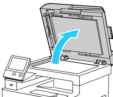
3. To access the jammed paper, open the Second-Side Scanning Access Cover, then remove any jammed paper.
