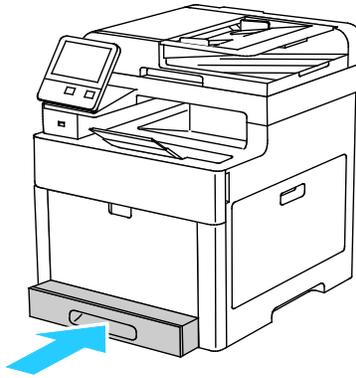
4. Load paper into the tray before inserting it back into the printer. For details, refer to [Loading Paper into Trays 1 and 2](#) on page 77.
