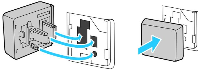
**⚠ CAUTION:** Pulling on the adapter can damage it. Once installed, remove the adapter only as needed, and according to the Wireless Network Adapter removal instructions. For details, refer to [Removing the Wireless Network Adapter](#) on page 44.
