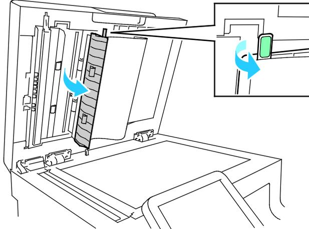
7. Using a soft cloth moistened with water, wipe the mirrored glass, the white-plastic strip, and the rollers. If dirt is difficult to remove, moisten a soft cloth with a small amount of neutral detergent, then wipe the printer parts dry with a soft cloth.
