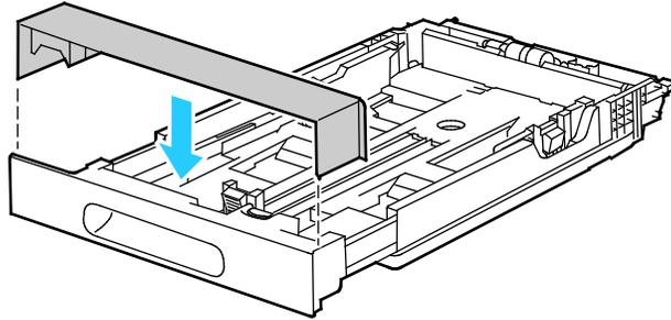
**Note:** If the tray is extended for Legal-size paper, the tray protrudes when it is inserted into the printer.
