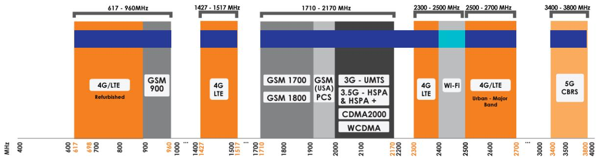
Indicates the LTE bands on which OMNI-414 works  Indicates the WI-FI bands on which OMNI-414 works
