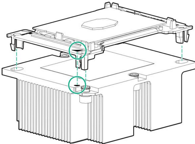
**11. Install the processor heatsink assembly.**
