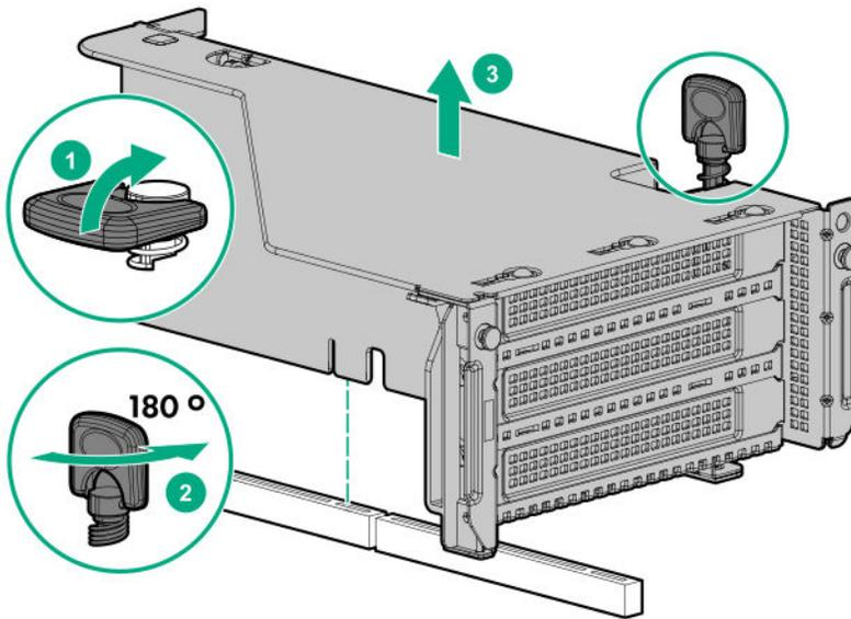
6. Identify and then remove the PCIe blank from the riser cage.
