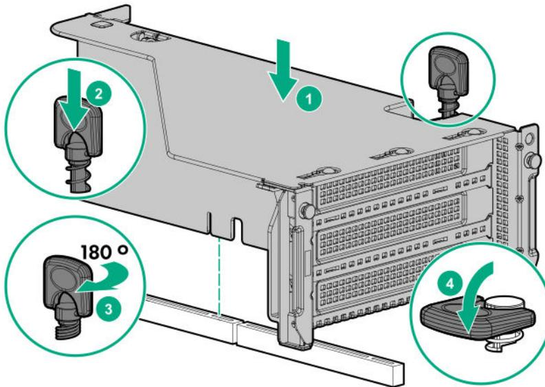
16. For full-length cards, slide the retention clips to the locked position.
