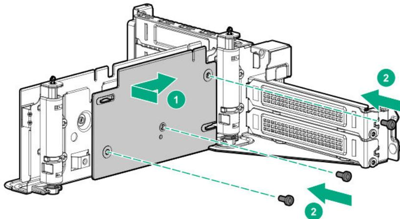
7. **If needed, install an expansion board.**
