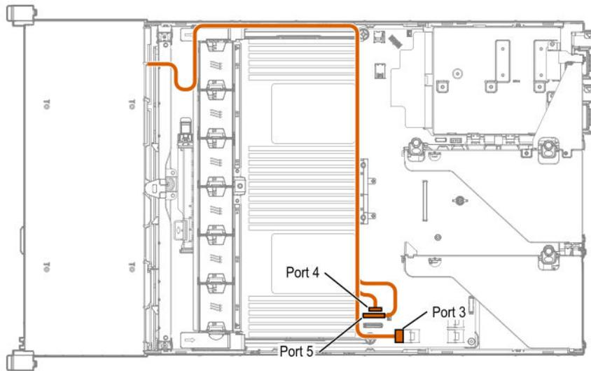
**Figure 2: Front 4LFF drive cage 1 (2SFF option)**
