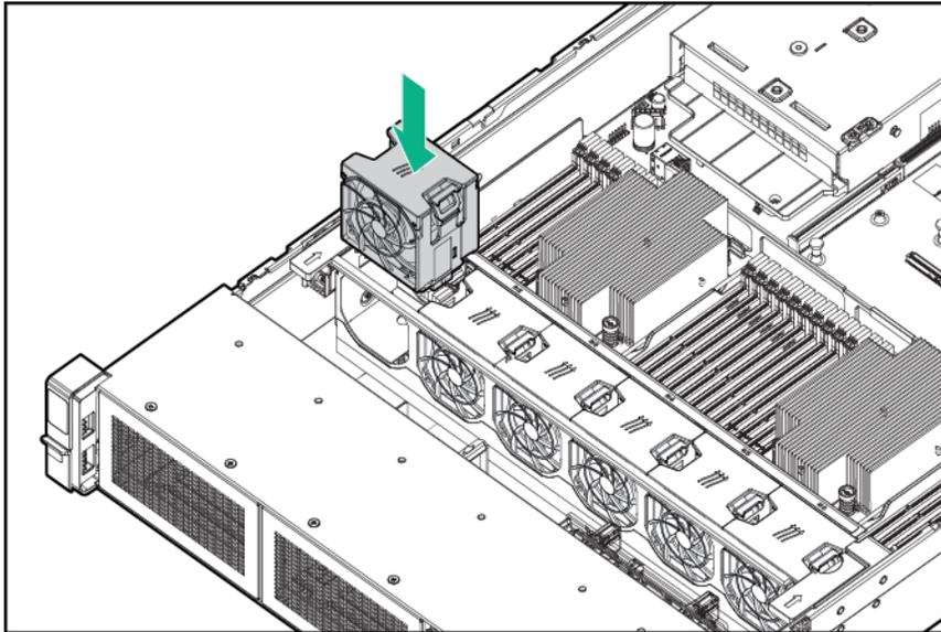
7. **Install the air baffle.**
