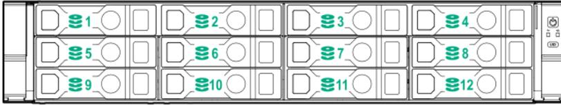
When any stacked 2SFF drive configuration is connected to the SAS expander, the drive numbering skips the second number to allow **uFF drive bay numbering**.
