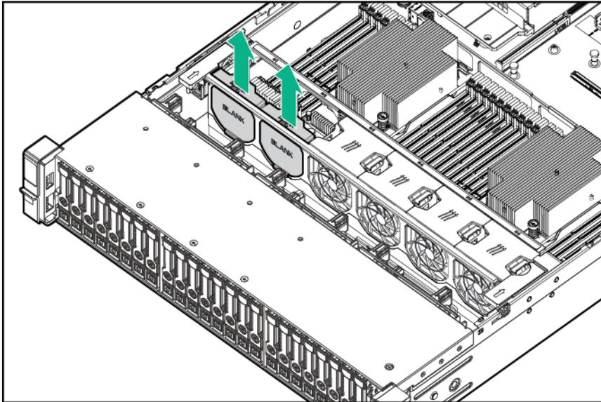
**4. Remove the air baffle.**
