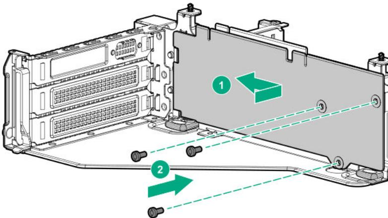
8. **If needed, install an expansion board.**
