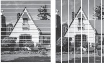
After the print head nozzle is cleaned, the lines are gone:
