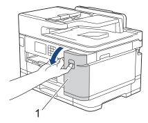
2. Press the lock release lever to release the ink cartridge colour indicated on the LCD and remove the ink cartridge from the machine, as shown in the illustration.
