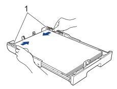
10. Make sure the paper is flat in the tray and below the maximum paper mark (1). Overfilling the paper tray may cause paper jams.
