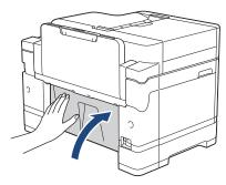
9. If your LCD displays [Jam Front/MP Tray] or [Repeat Jam Front/MP Tray], make sure you look carefully inside the MP tray for jammed paper. Push the release lever (1) towards the back of the machine, and then slowly pull the jammed paper out of the MP tray.
