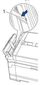
10. If your LCD displays [Jam Front/Manual Feed Slot] or [Repeat Jam Front/Manual Feed], make sure you look carefully inside the manual feed slot for jammed paper and slowly pull it out of the machine.
