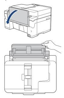
2. Slide the manual feed slot paper guides to fit the width of the paper you are using.
