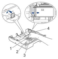
5. Load up to 20 sheets of photo paper in the paper tray with the printing surface **face down**. Loading more than 20 sheets of photo paper may cause paper jams.
