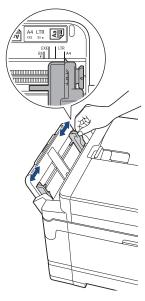
3. Load only **one sheet of paper** in the MP tray with the printing surface **face up**. Using both hands, push one sheet of paper into the MP tray until the front edge touches the paper feed rollers.
