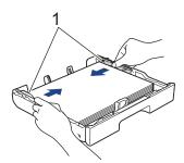
9. Make sure the paper is flat in the tray and below the maximum paper mark (1). Overfilling the paper tray may cause paper jams.
