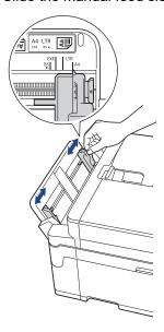
3. Load only one sheet of paper in the manual feed slot with the printing surface face up.
