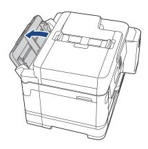
2. Gently press and slide the MP tray paper guides to match the width of the paper you are using.
