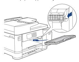
9. Replace the tray top cover and slowly push the paper tray completely into the machine.
