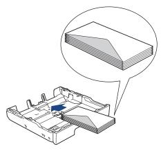
5. Gently press and slide the paper width guides (1) and paper length guide (2) to fit the size of the envelopes. Make sure the envelopes are flat in the tray.
