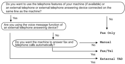
1. Press | Settings | > [All Settings] > [Fax] > [Setup Receive] > [Receive Mode].
