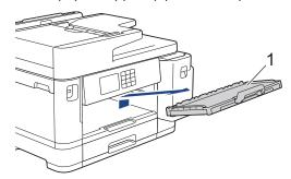
5. Clean the Paper Pick-up Rollers (1) with a soft lint-free cloth moistened with water. Slowly turn the rollers so that the whole surface is cleaned. After cleaning, wipe the rollers with a dry, soft lint-free cloth to remove all moisture.
