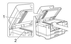
4. (MFC-J2740DW/MFC-J5740DW/MFC-J5955DW) Open the scanner glass cover (1), and clean the white bar (2) and the glass strip (3) with a soft lint-free cloth moistened with water.
