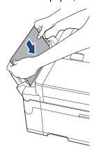
4. (MFC-J2740DW/MFC-J5740DW/MFC-J5955DW) Follow the instructions on the LCD to locate and remove the jammed paper.
