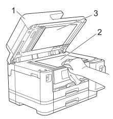
3. In the ADF unit, clean the white bar (1) and the glass strip (2) with a lint-free cloth moistened with water.
