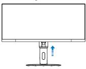
Place the monitor face down on a smooth surface. Pay attention not to scratch or damage the screen. Then lift the monitor stand.
