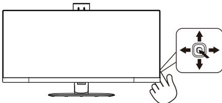
To access the OSD menu on this Philips Display simply use the single toggle button at the bottom of the Display bezel. The single button operates like a joystick. To move the cursor, simply toggle the button in four directions. Press the button to select desired option.
