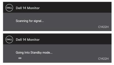
If USB Type-C cable is connected but without video signal, a floating dialog box as shown below appears.
