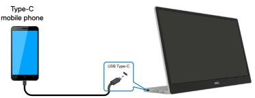
NOTE: For normal usage, devices of notebook and mobile phone that connect to C1422H need to support video signal and power output of 7.5W(5V/1.5A). When you encounter abnormal display condition, please check your devices to see if they support USB Type-C Alt-mode display and PD2.0 or above. After checking, please re-connect and try again.
