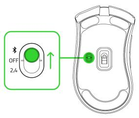
2. Press and hold the two side buttons, the DPI stage up, and the DPI stage down buttons simultaneously for three seconds to activate pairing mode. The status indicator will blink twice in repeated intervals to show that the device is in pairing mode.
