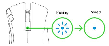
Once paired, your Razer DeathAdder V2 X HyperSpeed will automatically reconnect to your device whenever in Bluetooth mode and within range. Keep the pairing devices within close proximity of each other for faster and more stable connection.
