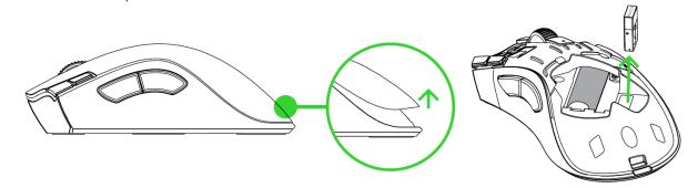
2. Close the top cover and insert the wireless dongle into any of the USB ports on your PC.
