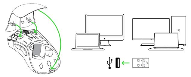
3. Push the slider switch to Razer<sup>™</sup> HyperSpeed Wireless (2.4 GHz) mode. When connected, the status indicator will briefly turn static green.
