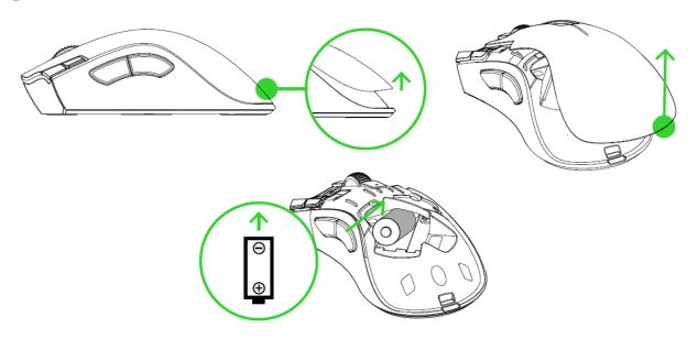
Caution: The included AA battery is non-rechargeable. Only one (1) battery will fit in the battery compartment. Do not forcefully insert two (2) batteries at the same time. Dispose batteries in accordance with your local environmental laws. For your safety, use only lithium or alkaline batteries.
