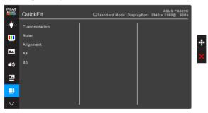
• Customization: You can decide the frame size by moving the ■ Menu (5-way) button up/down/left/right. You can press the ■ Menu (5-way) button for longer than 3 seconds to switch the measurements between millimeter and inch.
