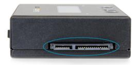
3. Connect your Target drive to the SATA SSD/HDD Target Port on the SATDUP11IMG.
