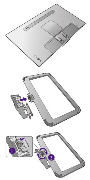
Orient and align the stand arm with the monitor, then push them together until they click and lock into place.
