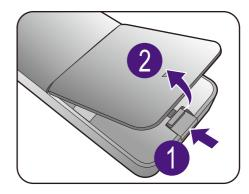
2. Press down the upper part of the battery so you can remove the battery from the lower part as illustrated.
