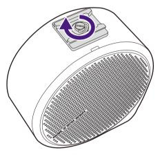
2. Install the projector onto the tripod.
