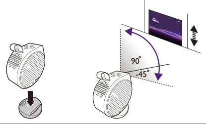
• The maximum angle of adjustment is 135 degrees.
