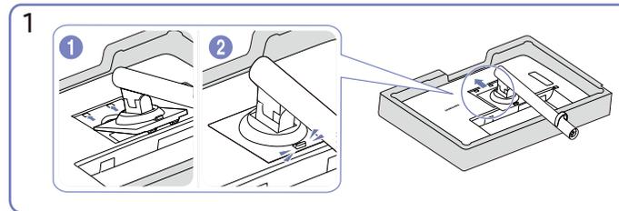
Push the assembled stand into the main body in the direction of the arrow as shown in the figure.
