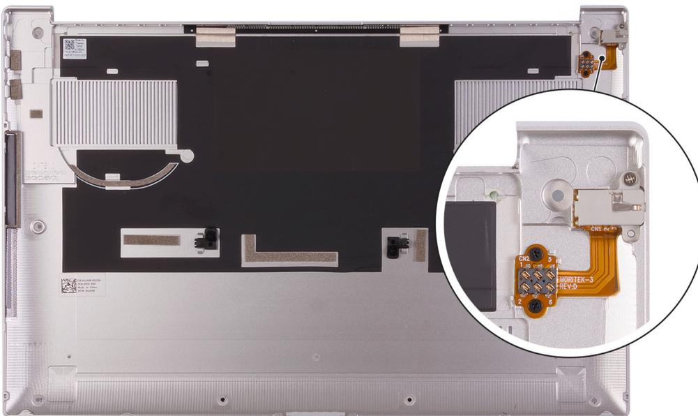
2. Starting from the bottom-left corner, use a plastic scribe to pry the base cover in the direction of the arrows to release the base cover from the palm-rest and keyboard assembly.
