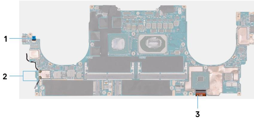
**Figure 2. System-board connectors**
