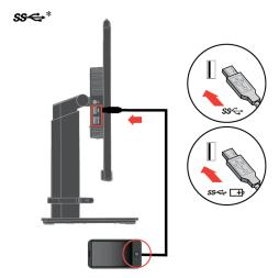
**Note:** The USB Battery Charging port (with battery symbol) specification 1.2 output 5Vdc/1.5A (typical), 2A (max) and the other standard USB Output 5Vdc/900mA. The USB downstream port does not provide power while the monitor is switched off.
