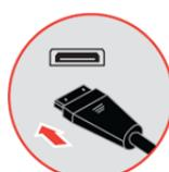
4. Connect one end of the USB 3.0 cable to the USB connector on the back of the computer, and the other end to the upstream USB connector on the monitor.
