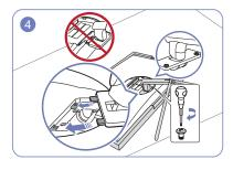
Fasten the screws at the bottom of the stand neck.
