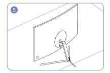
Tide up the connected power supply and the data cable then cover the COVER-REAR SUB as shown in the figure.
