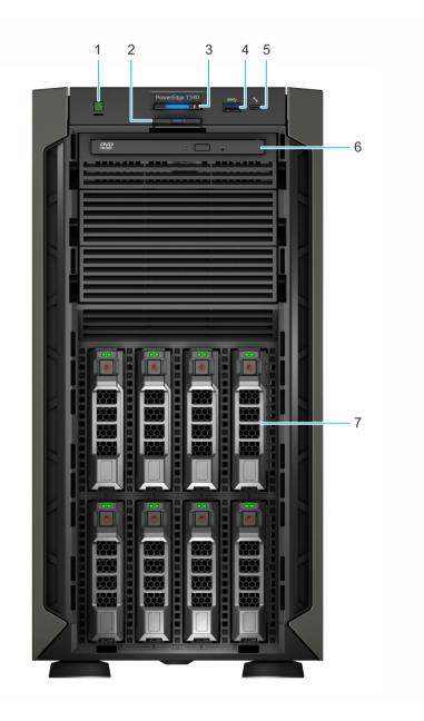
Figure 1. Front view of  $8 \times 3.5$ -inch drive system
