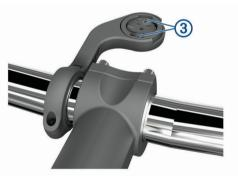
7 Press down slightly and turn the Edge device clockwise until it locks into place.
