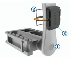
4 Rotate the crank arm to check for clearance. The sensor and bands should not contact any part of your bike or shoe.
