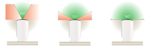
Each setting auto corrects the image to reduce the fisheye effect. The Full setting completely eliminates the fisheye effect.
