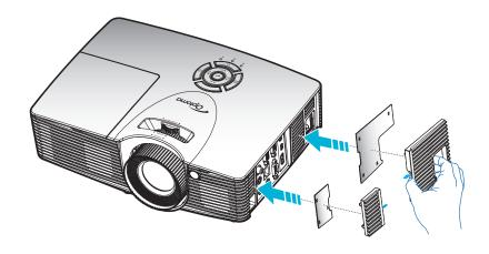
Note: Dust filters are only required/supplied in the selected regions with excessive dust.
