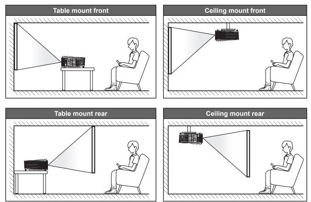
Projector should be placed flat on a surface and 90 degrees / perpendicular to the to the screen.
