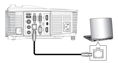
2. On the PC (Laptop), select Start > Control Panel > Network Connections.
