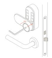
Step 7. Holding the Glue Smart Lock against the door, screw the two screws behind the battery cover to the door plate. Use the thumb turn on the Glue Smart Lock to check the deadbolt opens and closes smoothly, if not, return to Step 4 and check all parts are correctly fitted.
