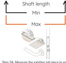
Step 3A. Measure the existing tail piece in your lock with the guide above. The end of the tail piece should not exceed the max line.
