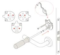
Step 4. Use screws from step 2 to loosely attach the door plate. Use holes shown above depending on the chosen mounting angle. The rubber side of the plate faces the door. If a different length screw is required, cut the longer screws supplied to the correct length.
