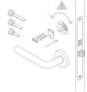
Step 3C . Replace with one of the three tail pieces supplied, choose one that fits between the MIN and MAX lines (step 3A).
