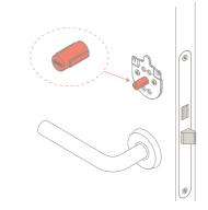
Step 5. Slide the insert supplied over the tail piece.
