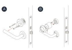
Step 2A. Remove the existing inside thumb turn by unscrewing the two screws in the thumb turn plate. Follow step 3A.
