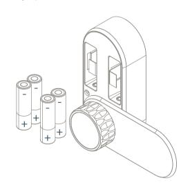
To replace the batteries rotate the front cover of the product and pull the fabric tabs to release your existing AA batteries..
