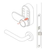
Step 8. Check the lock is securely fastened to the door. If not, check all screws in step 4 and then step 7 are tightened. Then remove the battery tabs. The light behind the thumb turn will flash.
