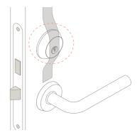
Step 1. Download the latest GLUE LOCK App. Secure the lock cylinder on the outside of the door with sticky tape. This makes it easier whilst you fit your Glue Smart Lock.
