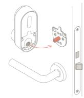
Step 6. Turn the thumb turn on the Glue Smart Lock to the approximate centre, until the slots inside the turning section align with the ribs on the insert. Then slide the Glue Smart Lock over the insert onto the door plate.
