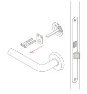
Step 3B. If the tail piece is too short, or too long, unscrew the D-plate and carefully remove it. Be careful not to drop the screws inside the door body.
