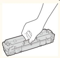
To avoid scratching the surface ( [a]) of the drum inside the machine or exposing it to light. Do not touch the electrical contacts ( $\bigcirc$ ) or the toner cartridge memory ( $\bigcirc$ ).
