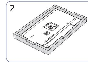
Place the protective Styrofoam (cushion) included in the package on the floor and place the product facing down on the Styrofoam, as shown in the image. If Styrofoam is unavailable, use a thick sitting mat.
