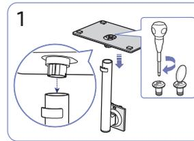
Put the stand base onto the stand neck as the direction shown in the figure. Tightly fasten the connecting screw at the bottom of the stand base.
