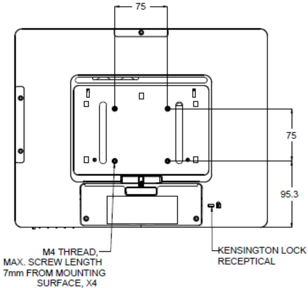
For the 17-inch touchmonitor, a four-hole 75x75mm mounting pattern for M4 screws is provided on the rear of the monitor. Remove the stand using a Phillips screwdriver to access this mounting interface. The VESA FDMI-compliant counting is coded: VESA MIS-B, 75, C.
