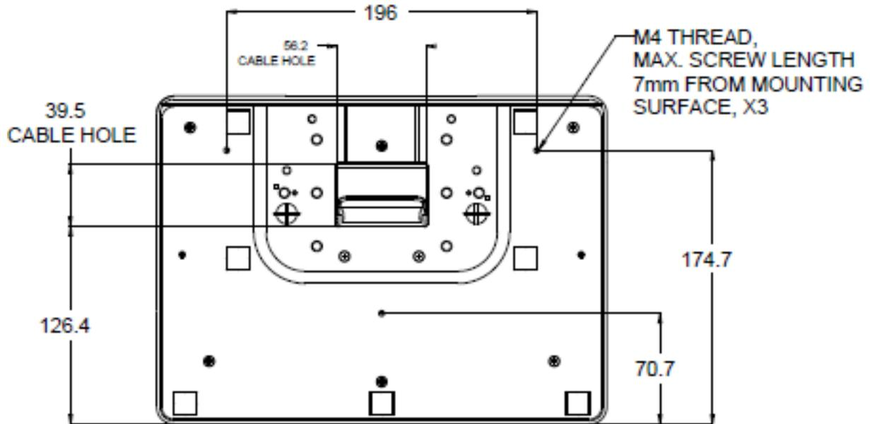
For the 17 inch touchmonitor, a threaded three-hole mounting pattern for M4 screws is provided on the bottom of stand base for mounting or securing.
