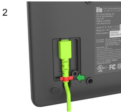
2 Connect the micro USB cable. Ensure the rubber gasket (red) is all the way inside the cable cover area.
