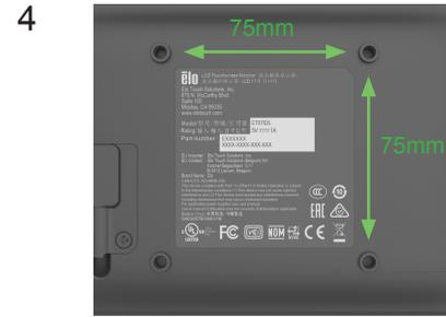
4 Monitor can be mounted to any standard 75mm x 75mm VESA mounting bracket using four M4x8mm screws.
