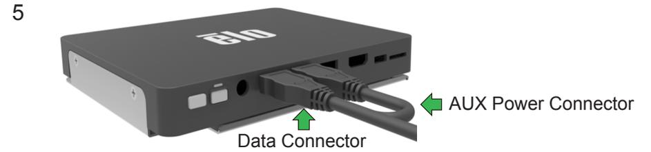
5 Connect the Data Connector of the Y-Cable to the host PC USB port. Note: Some computers also require connecting the AUX Power connector to the host PC.
