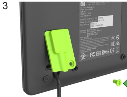
3 Install the cable cover by installing the top side first and rotating it down. Secure the door with the M3 screw included.
