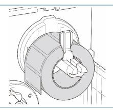
Push the Print Head Release Lever and thread the label through the Damper, Media Sensor, and Front Label Guide to install the media.
