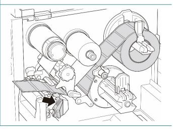
5. Move the Media Sensor by adjusting the Media Sensor Position Adjustment Knob. Make sure the position of the Gap or Black Mark Sensor matches the position of the Gap/Black Mark on the label roll.
