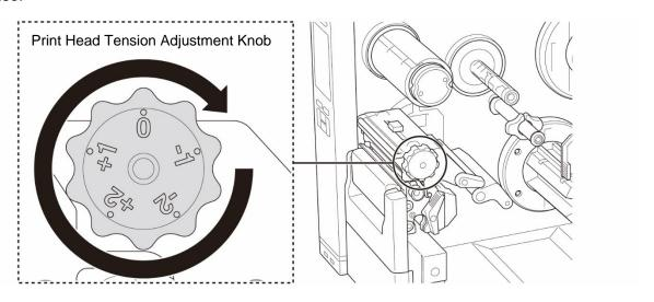
For labels (less than 2" width), set the Print Head Tension Position Adjustment Slider as close to the label edge as possible to prevent unnecessary friction between the Print Head and the Platen Roller.
