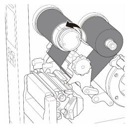
6. Close the Print Head by pushing down on both sides of the Print Head Release Lever.
