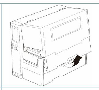
2. Slide the Label Roll Guard horizontally to the end of the Label Supply Spindle, and then flip down the Label Roll Guard.
