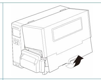
2. Slide the Label Roll Guard horizontally to the end of the Label Supply Spindle, and then flip down the Label Roll Guard.
