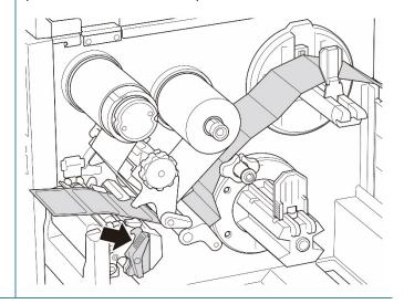
4. Move the Media Sensor by adjusting the Media Sensor Position Adjustment Knob. Make sure the position of the Gap or Black Mark Sensor matches the position of the Gap/Black Mark on the label.
