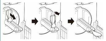
Place the label roll on the Label Supply Spindle and then flip the Label Roll Guard upwards to hold it in place.
