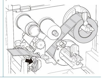
5. Move the Media Sensor by adjusting the Media Sensor Position Adjustment Knob. Make sure the position of the Gap or Black Mark Sensor matches the position of the Gap/Black Mark on the label roll.
