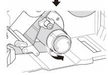
14. Lock the Print Head Release Lever and set the print mode to "Peel Off" using the Main Menu.
