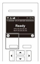
To select an option on the Main Menu, use the Navigation buttons to browse the options and then press the button under the  $\bigcirc$  icon.
