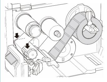
11. Close the Print Head and press the right **Selection** button to feed one label to test.
