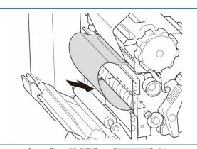
13. Wrap the liner around the paper core and adhere the liner to the Media Rewind Spindle. Wind the liner on the Media Rewind Spindle until the liner is fully stretched.
