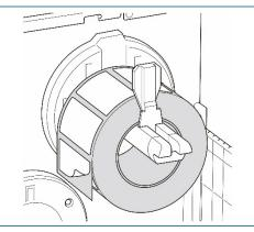
Push the Print Head Release Lever and thread the label through the Damper, Media Sensor, and Front Label Guide to install the media.
