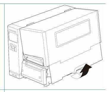
Slide the Label Roll Guard horizontally to the end of the Label Supply Spindle, and then flip down the Label Roll Guard.
