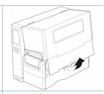
2. Install the ribbon onto the Ribbon Supply Spindle.
