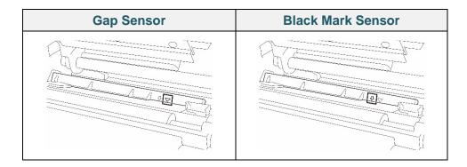
The Gap Sensor (transmissive sensor) detects the beginning of the label and the printer feeds the label to the correct position.
