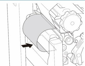
14. Wrap the label around the internal Media Rewind Spindle and adhere the label to the Paper Core. Wind the spindle counterclockwise until the label is fully stretched.
