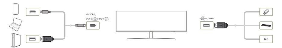
If multiple devices are connected to a source device, the many cables around the source device may look messy. Connecting the devices directly to the product will resolve such inconvenience.
