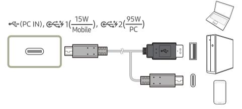
Connect the USB cable to on the back of the product and to on the source device.
