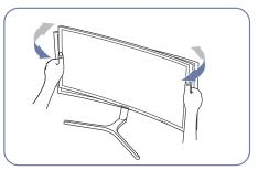
• Grasp the left and right sides of the monitor and adjust the tilt.
