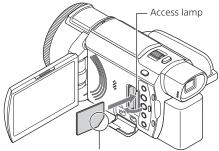
Insert the card with the notched corner in the direction as illustrated.
