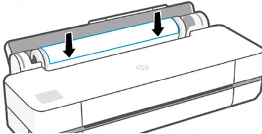
5. Roll the paper into the printer until you feel resistance and the paper flexes slightly. When the printer detects the paper, it beeps, and feeds in the paper automatically.
