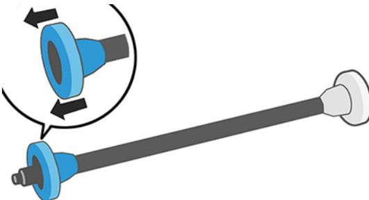
3. If the roll is long, rest the spindle horizontally on a table and load the roll on the table.
