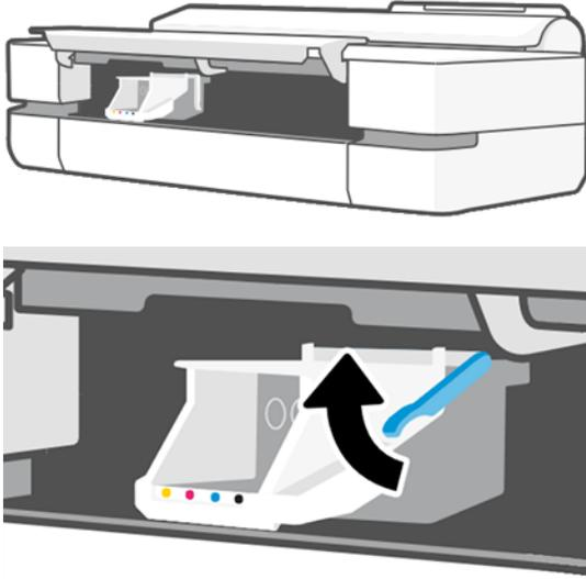
9. Remove the printhead, keeping it vertical to avoid getting ink on the connections.
