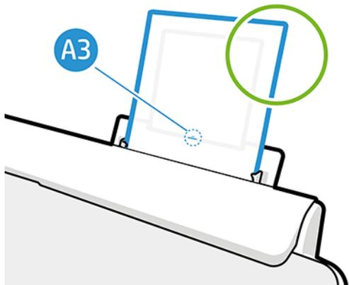
If the paper is hanging over the back of the input tray as shown, it may fail to load.
