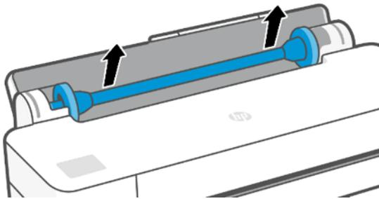
2. The spindle has a stop at each end to keep the roll in position. The blue stop can be removed to mount a new roll; it slides along the spindle to hold rolls of different widths. Remove the blue paper stop from the end of the spindle.
