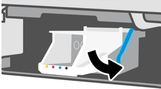
12. Insert the ink cartridges. Make sure that you insert each ink cartridge into the slot that has the same colored label as the cartridge you are installing.
