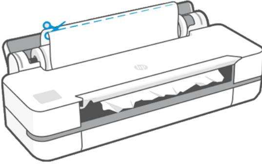
4. Carefully remove any of the jammed paper that you can from the top of the printer.
