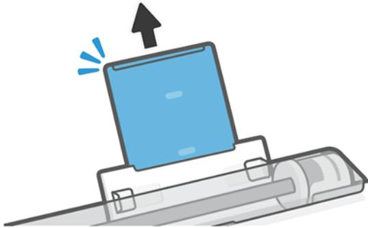
3. Load sheets of paper into the tray with the printed side facing outwards. Ensure that the sheets are all of the same size.
