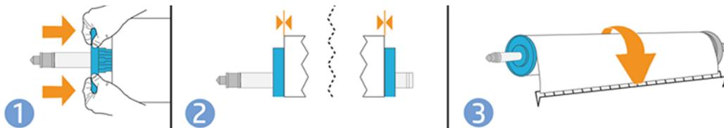
6. Ensure the blue paper stop is pushed in as far as it goes. Check that there is no space between the roll and the stops at both ends.
