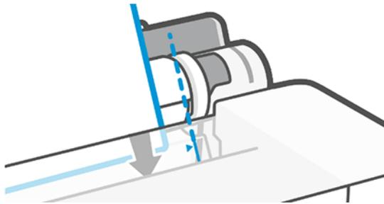
7. Tap **OK** on the front panel to feed the paper into the printer. Guide the sheet into the printer; this is especially important with thicker papers.
