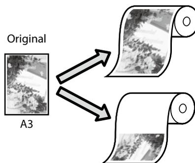
Fitting the short side of the original to the roll paper width.
