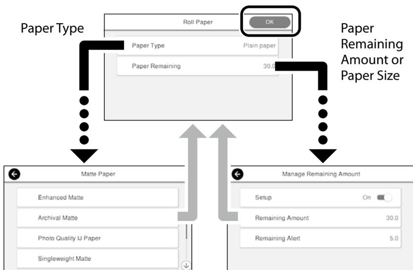
Promptly select the settings because the paper will start being fed if the screen is not used for 90 seconds.
