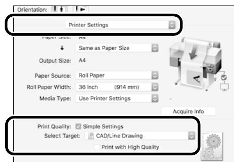
Print CAD and GIS drawings using either of the following two methods depending on the intended use of the drawing.
