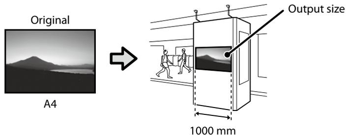
Select **Output Size - Fit to Output Size**, and then select the output size.
