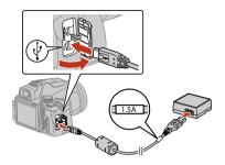
2 Insert the plug of the Charging AC Adapter into an electrical outlet.
