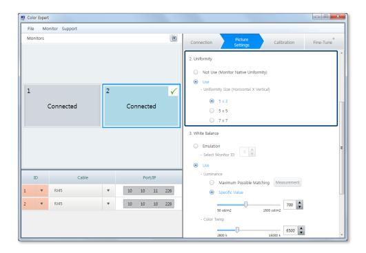
**Uniformity Size** (Horizontal X Vertical) Specify the number of columns and rows to split the screen you want to calibrate the uniformity for.
