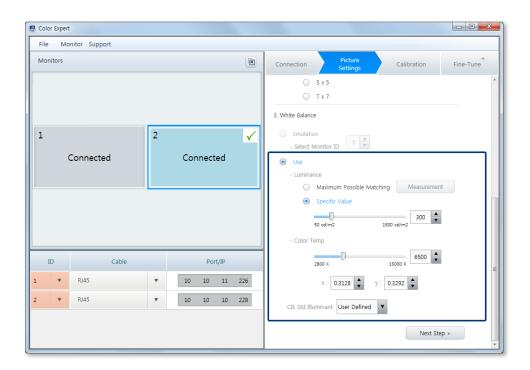
Specify the target brightness. • Maximum Possible Matching: Measure and apply the maximum brightness available on the LFD. To measure the brightness, click Measurement. Luminance • Specific Value: Manually enter a desired brightness level. A higher value increases the screen brightness. The range of available luminance levels may vary depending on the LFD model.
