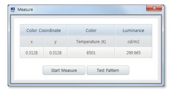
Luminance and color temperature results can vary after calibration, depending on the input source (DisplayPort or HDMI). If this is the case, adjust the HDMI signal output level or check HDMI Black Level for the LFD screen.
