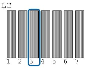
The screen to enter a numeric value is displayed. Enter the value for each check pattern number (such as #1) and ink color that you checked in step 9, and then press the OK button.
