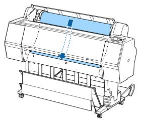
17 With both hands, pull the roll paper until the leading edge of the paper is in the center of the stand (the position of the label shown in the illustration).
