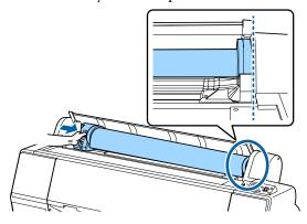
Raise the lock levers on the adapter holders to lock them in place.
