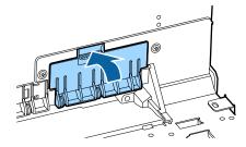
After replacing the cutter, press the **OK** button. The cutter will return to its original position.
