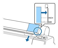
For paper smaller than A4 size, insert by keeping the right edge aligned with the additional line below the paper feed slot.
