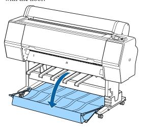
Lower the paper supports while pressing the left and the right sides until the supports are vertical as shown in the illustration.
