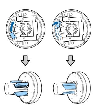
Raise the adapter lock lever to release the lock on each of the two roll paper adapters.
