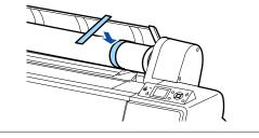
Lower the lock lever for the adapter holder to release the lock.
