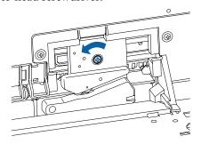
Remove the old cutter from the printer.
