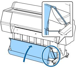
When the cloth touches the floor, secure using the hook and loop fastener tape as shown in the illustration.
