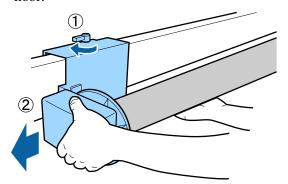
Remove the roll core from the auto take-up reel unit.
