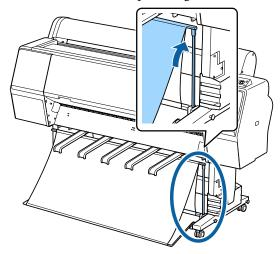
Lower the paper supports while pressing left and right as shown in the illustration until they touch the cloth.
