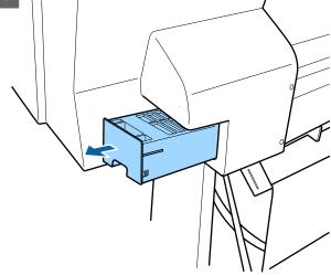
Place the used maintenance box in the clear bag included with your new maintenance box, and make sure that the zipper is closed tight.
