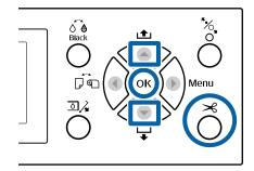
With the front cover closed, hold down the ▼ button on the control panel while viewing the inside of the printer until the cutting position reaches the position of the label.
