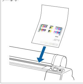
Position the trailing and right edges of the paper as shown by the loading mark.
