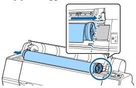
Move the adapter holder so that the ▲ on the adapter holder and the left roll paper adapter are aligned.
