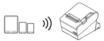
SimpleAP mode is enabled by default when shipping from the factory. When SimpleAP mode is enabled and the printer is turned on, the following information is printed automatically.
