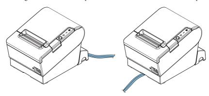
After the cable arrangement, turn over the printer, and make sure the cables are not pinched.
