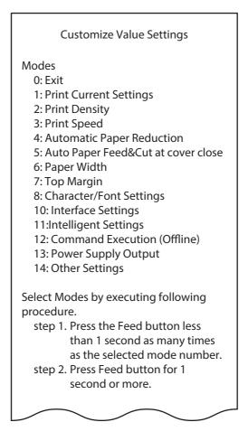
**3** After briefly pressing the Feed button (less than one second) for the number of times shown in the print result, hold down the button for more than one second to select the setting items.
