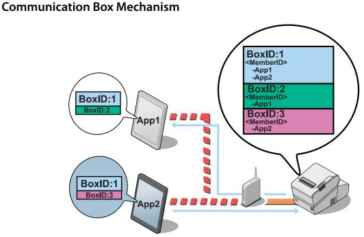
The TM-Intelligent software manages the communication box with a box ID (BoxID in the figure above). Data can be exchanged between applications that belong to the communication box.
