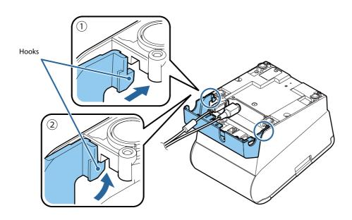
**3** Push the connector cover down to click onto the printer case.
