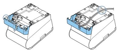
When using cables without lock, use of the bundled cable lock band is recommended.
