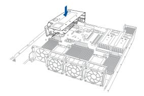
9. Secure the riser card bracket 1 to the chassis with the screw removed in step 1.
