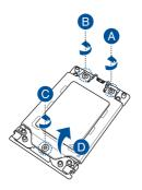
4. Slightly lift open the rail frame.
