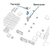
Select an appropriate screw hole on the motherboard for your M.2 card, then secure the stand to the motherboard.
