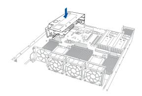
6. Secure the riser card bracket 1 to the chassis with the screw removed in step 1.
