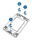
9. Twist each of the four screws with a Phillips screwdriver just enough to attach the heatsink to the motherboard. When the four screws are attached, tighten them one by one in a diagonal sequence to completely secure the heatsink.
