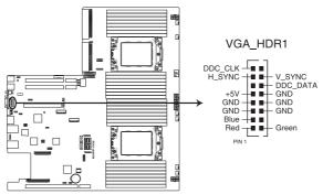
**KNPP-D32 Internal VGA connector**
