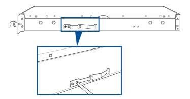
Select a desired space and place the appropriate rack rail (left and right) on opposite positions on the rack.
