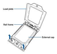
5. Slide the external cap out of the rail frame.
