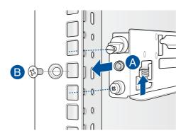
8. Lift the server chassis and insert it into the rack rail.
