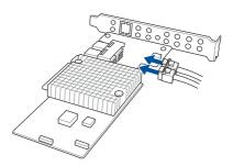
7. Install the replacement ASUS PIKE II card into the riser card bracket 1 (A), then secure it with the screw (B).
