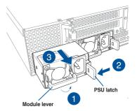
Insert the replacement power supply module into the chassis then push it inwards until the latch locks into place.
