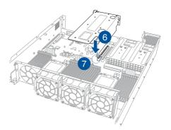
8. Secure the riser card bracket 2 to the chassis with the screws removed in step 1.
