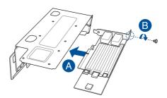
Install the riser card bracket 3 and the PCIE expansion card assembly into the PCIE4 slot on the motherboard. Ensure that the golden connectors of the riser card bracket 3 is firmly seated in place.
