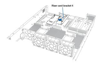
Move the metal lock downward to secure the riser card bracket 4 and the PCIE expansion card assembly to the chassis.
