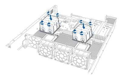
10. Reinstall the air ducts then secure the air ducts with the screws removed in step 2.
