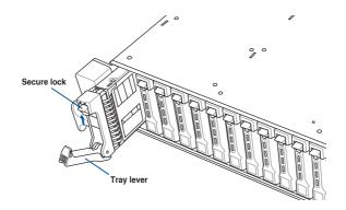
2. Firmly hold the tray lever and pull the storage device tray out of the bay.
