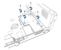
8. Reinstall the metal cover (A) and secure it with the screw (B).
