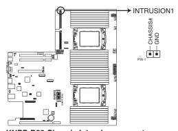
**KNPP-D32 Chassis Intrusion connector**
