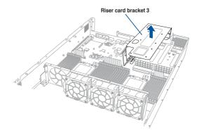
Remove the screw from the metal cover (A), then remove the metal cover (B) from the riser card bracket 3.
