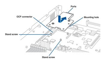
Secure the Mezzanine card with four bundled screws.
