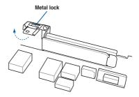
4. Remove the metal cover from the chassis.
