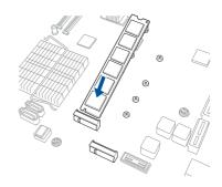
6. Secure the M.2 card with the top screw.
