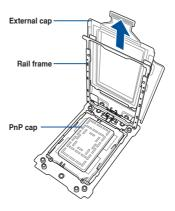
6. Slide the carrier frame with CPU into the rail frame, then remove the PnP cap.
