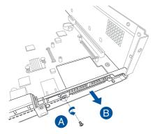
Select the slots that are going to be used for your Mezzanine card, then use a screwdriver and pry the corresponding slots until it pops off.
