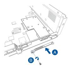
Install the riser card bracket 1 into the PCIE connector on the motherboard. For more information, refer to section 2.5.1 Installing an expansion card to riser card bracket 1.
