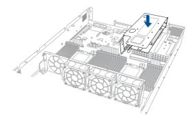
6. Secure the riser card bracket 3 to the chassis with the screws removed in step 1.
