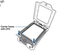
Close the load plate just enough to let it sit on top of the CPU, then secure each screw one by one in the sequence shown on the socket to completely secure the load plate.
