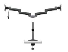
8. Place the dual mount (2) and the attached LCD arms (1) attached onto the pole.
