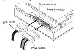
Figure 1 Attaching SATA cabling
